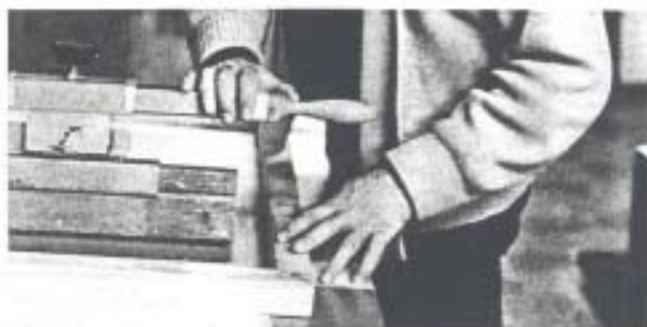
After the image is drawn on a screen, glue is painted around it to fill the screen holes in the non-image areas. Here, ink is being forced through the open-mesh holes in the image area with a rubber squeegee, transferring the image onto the sheet of paper below.
